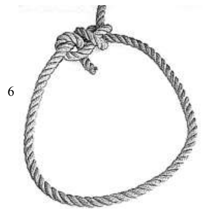
A bowline with a half hitch added as an extra safety measure.
